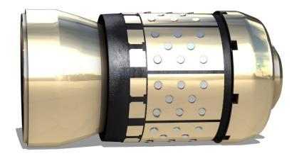
The Kronos™ dissolvable isolation tool is a revolutionary pump-down baffle that dissolves in low temperature, low salinity, or even fresh water wellbore environments. Like the plug and perf method, it is placed in the casing string using a conventional Baker or Go Shorty Hydraulic Setting Tool on wireline. This patent-pending tool is the latest technology developed by Peak Completions.
